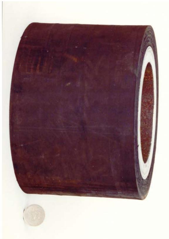
**Figure 4 Section of 6-inch nb flowline with 25 mm EPDM rubber coating**
