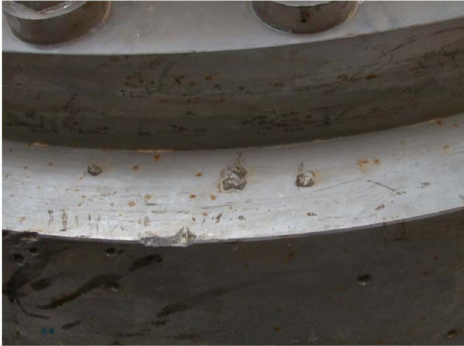
**Figure 5 Pitting damage to a stainless steel propeller hub – fast ferry newbuilding**
