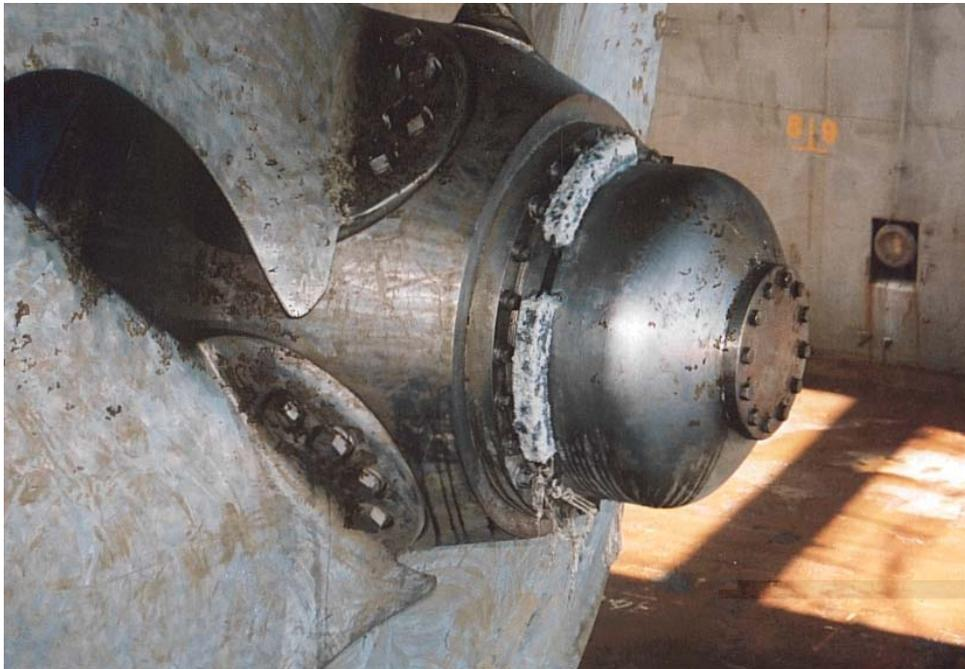
**Figure 6 sacrificial anodes to protect stainless steel propeller during outfitting**
